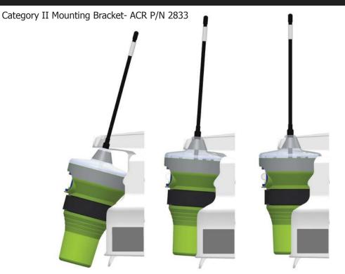
To mount the EPIRB in the category II bracket, insert the top cap first at a slight angle and then press the bottom casing until the EPIRB clicks and is firmly supported. The EPIRB can only be mounted inside the bracket with the ON/Test buttons facing out.
