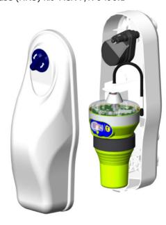
To mount the EPIRB in the category I bracket, insert the top cap first at a slight angle and then press the bottom casing until the EPIRB clicks and is firmly supported. The EPIRB can only be mounted inside the bracket with the ON/Test buttons facing out.
