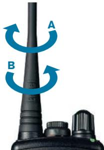
1. To attach, carefully align the antenna with the socket. Screw in the antenna clockwise (taking care not to cross the thread) until it is seated firmly with the accessory cover's rubber ring between the antenna and the top of the radio (A).
