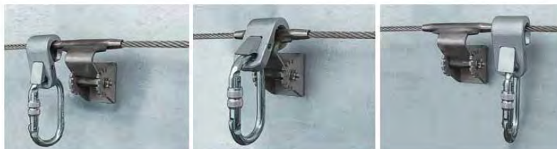
Sequence for travelling the slide, a movable anchor point, along the system including passing through a lug without hampering the fall protection capability
